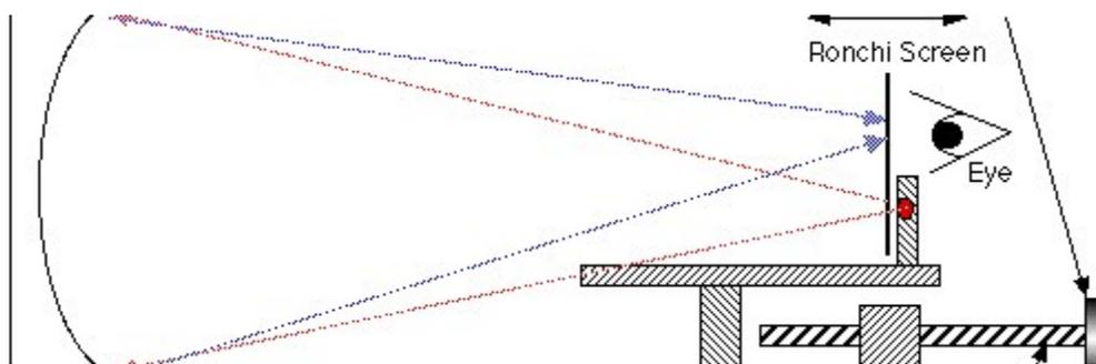
The mirror is on the left. Light leaves the bulb travels to the mirror and is reflected back to the observer who sits at the tester. It is important to have the tester on a solid table, as measurements for Foucault require accuracy to at least .002". Amazingly enough, get such accuracy is not too difficult to do even with common screws!
