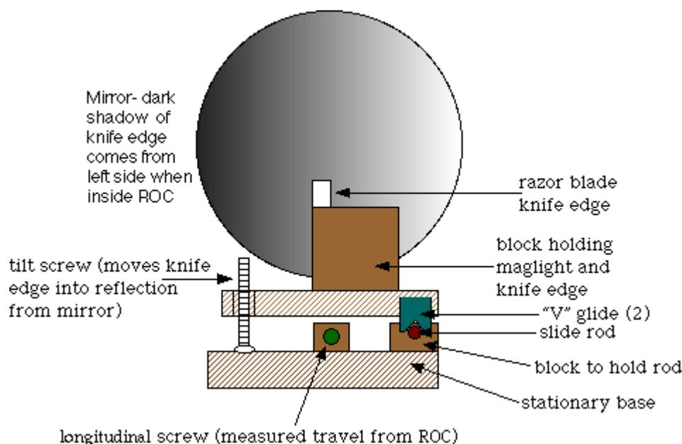
To perform the Foucault test or to adjust the Ronchi bands to appear where desired, the tilt screw is used to tip the entire top portion of the platform, as seen below:
